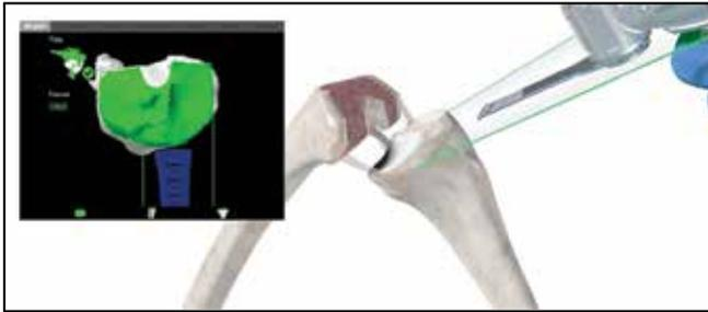
In the operating room, your surgeon guides Mako's robotic arm to remove the arthritic bone and cartilage from the knee. A virtual boundary provides tactile resistance to help protect soft tissue and help the surgeon stay within the boundaries defined in your surgical plan.
